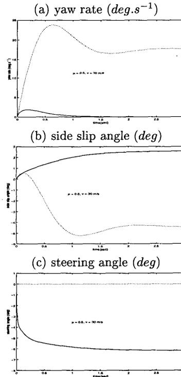
Figure 8: Wind force step input rejection for  $v = 30m.s^{-1}$  and  $\mu = 0.5$
