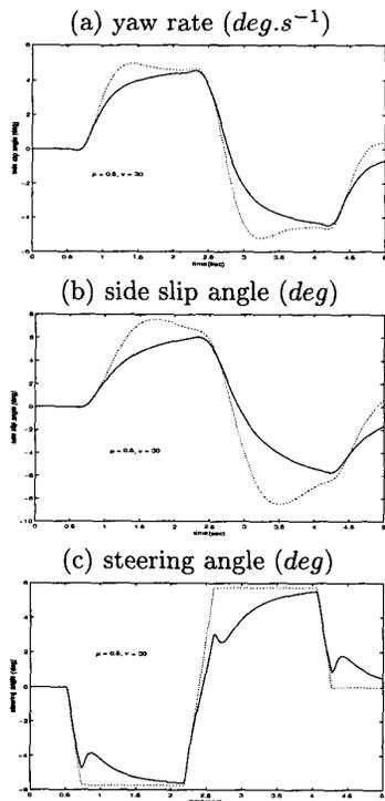
Figure 10: Lane change maneuver for  $v = 30m.s^{-1}$  and  $\mu = 0.5$
