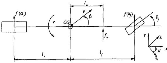
Figure 1: Lateral model data of the vehicle
