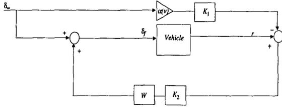
Figure 6: Active steering controller implementation
