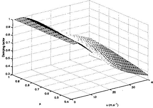
Figure 2: Damping factor function of speed and road adhesion
