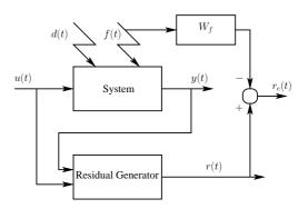
Fig. 1. Scheme of robust residual generation
