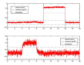
Fig. 2. Faults and corresponding residual signals
