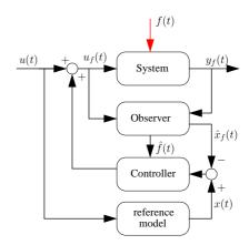
Fig. 1. Fault tolerant control scheme
