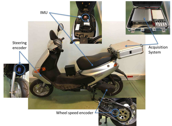
Fig. 1. Instrumented Scooter
