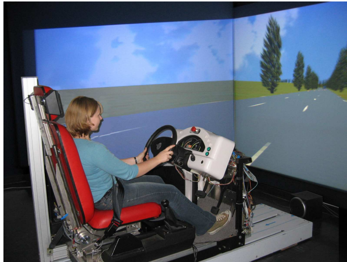
Figure 1.11. Mini-simulateur INRETS/IBISC - France.
